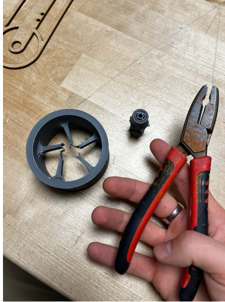
Figure 9: Empirical destructive torsion test performed on wheel prototype using pliers.
